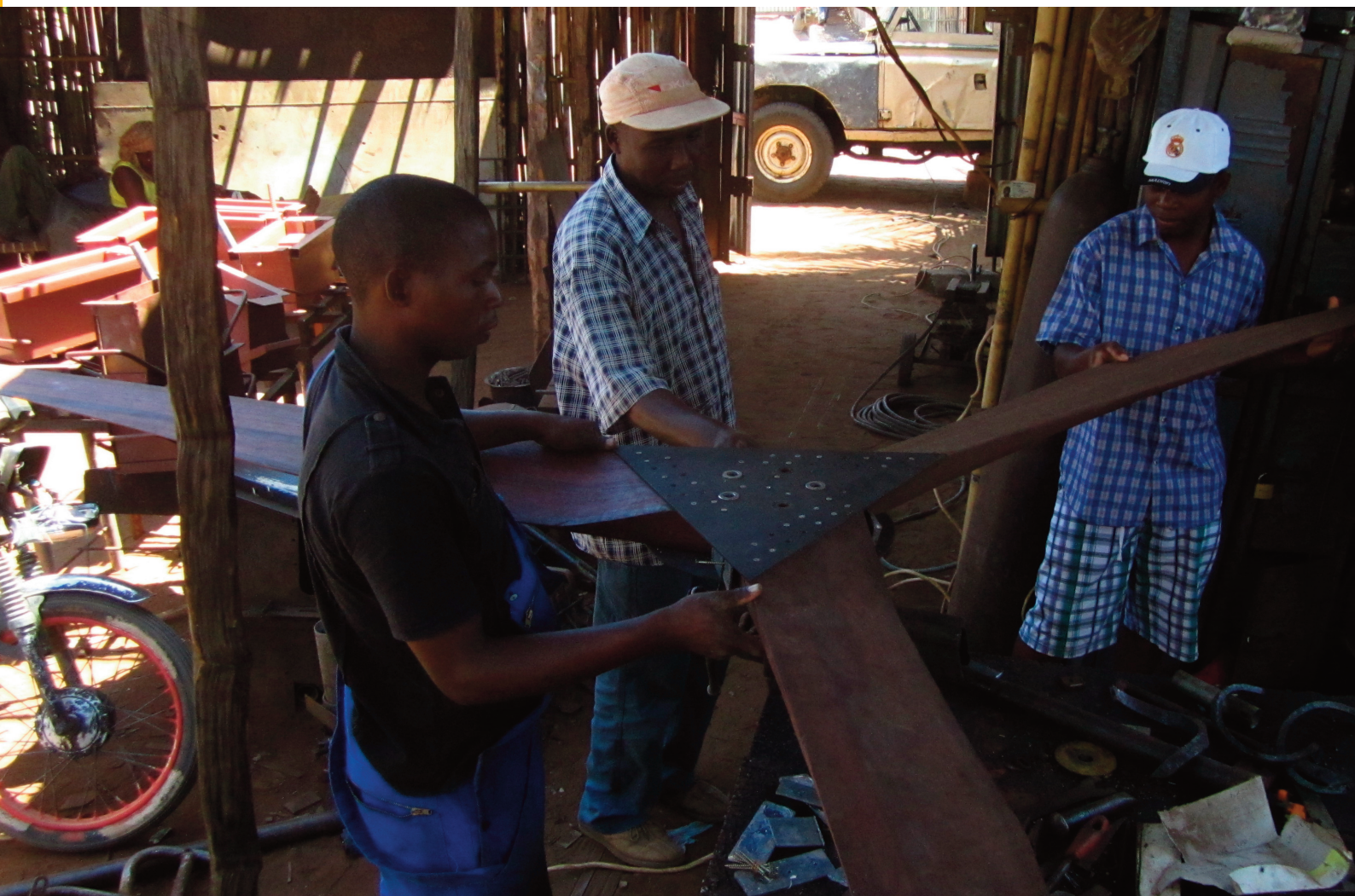
Image 5: Wind Blade Manufacturing, Pemba Source: www.renewable-world.org
