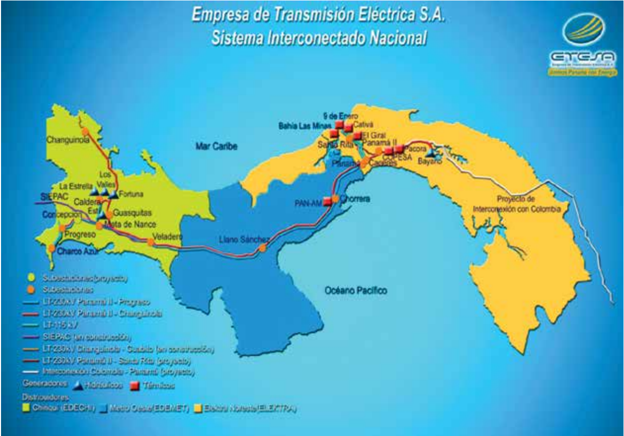
Figure 14: Transmission and distribution system in Panama
