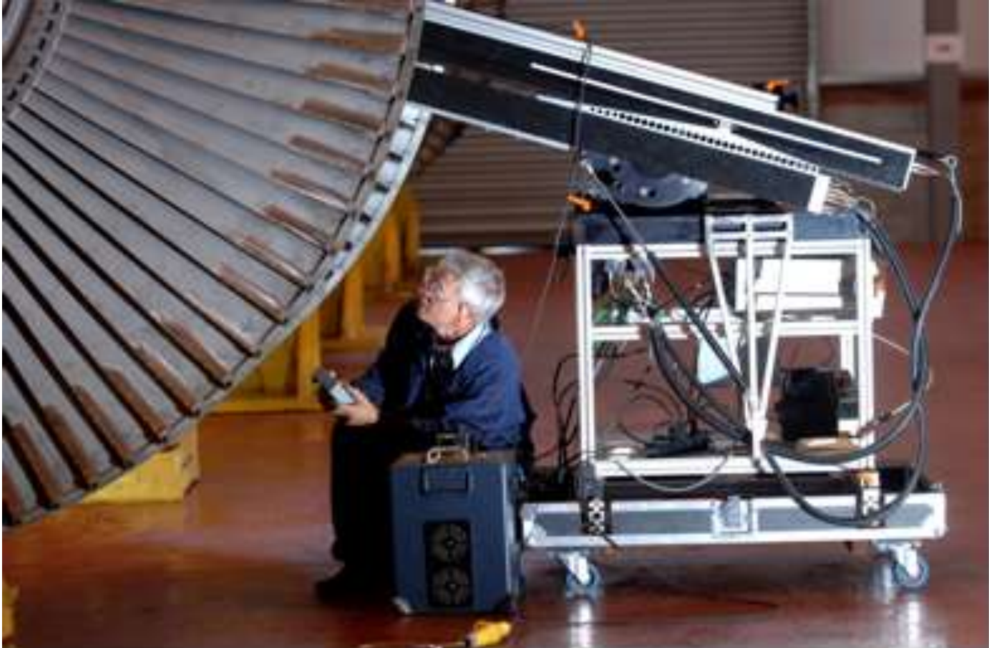
Inspection of turbine blade quality
