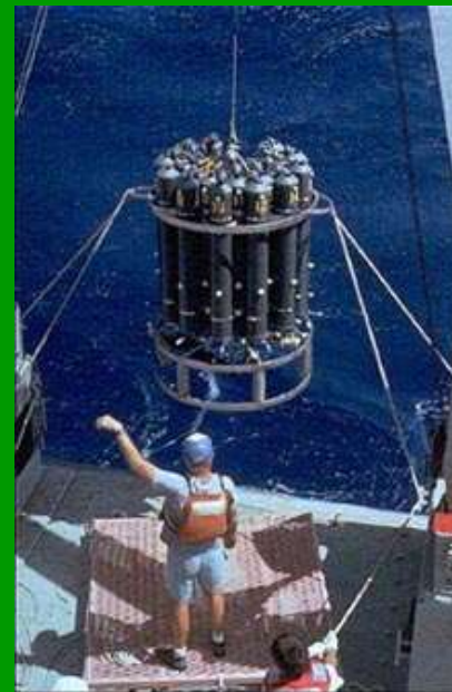
CTD (Conductivity-Temperature-Depth) package, combined with water sampling bottles and specialized sensors
