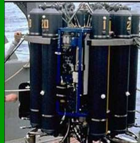
CTD (Conductivity-Temperature-Depth) package, combined with water sampling bottles and specialized sensors
