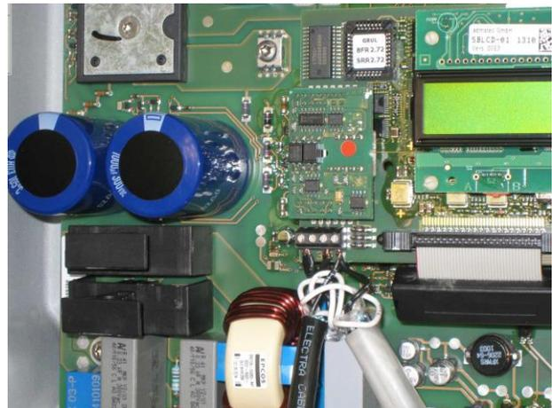
Wiring the data cabling in the inverter
