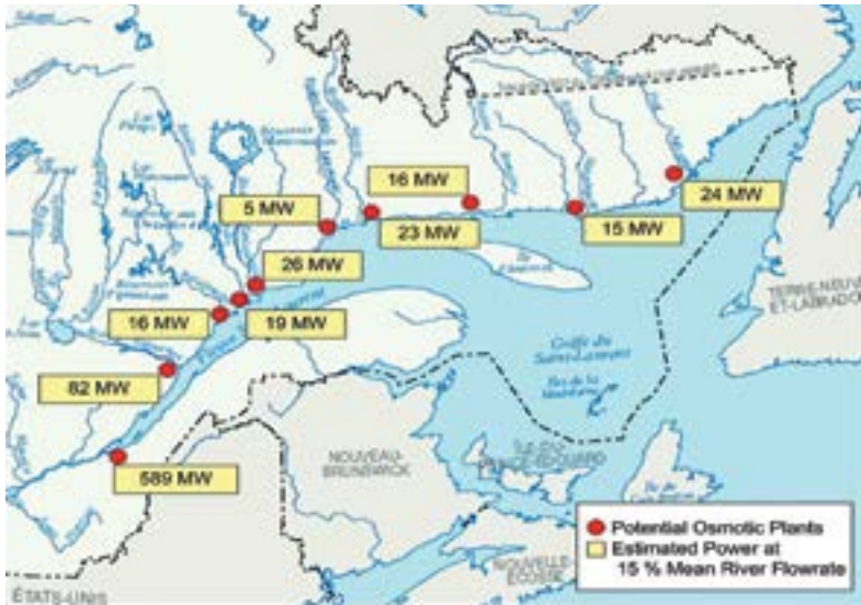
Figure 5: Sites for Osmotic Power Production along the Lawrence River based on a preliminary resource assessment.
