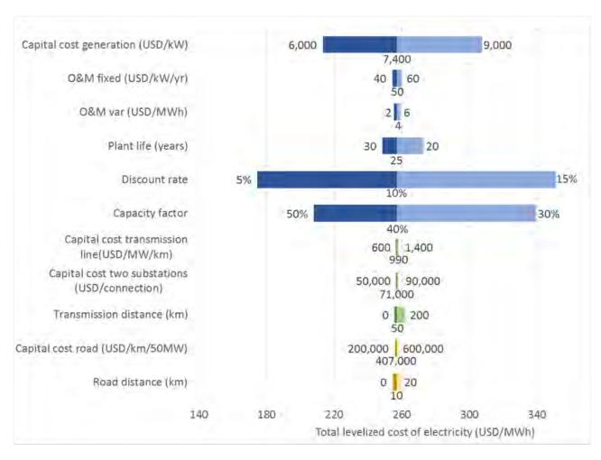
FIGURE 40: Total levelized cost of electricity (LCOE) sensitivity analysis for Solar CSP.
