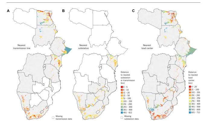
**FIGURE 29:** Comparison of distance to nearest transmission (A) and substation (B) with distance to nearest load center (C) for wind zones.
