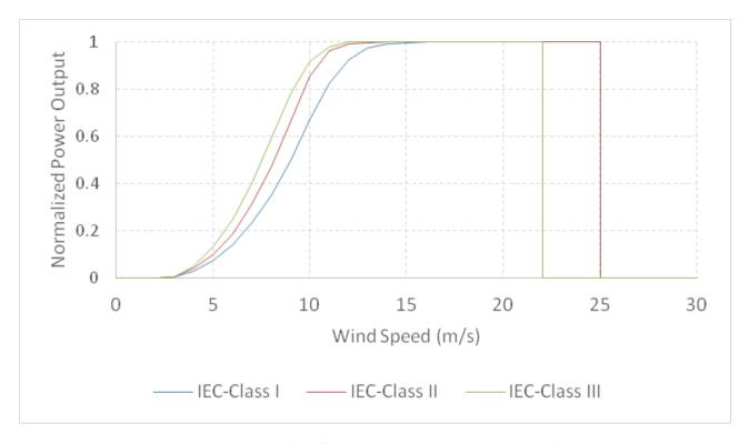
FIGURE 6: Normalized power curves for different IEC class turbines reproduced from [King et al., 2014].
