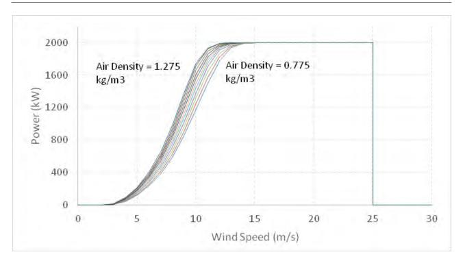
**FIGURE 7:** Adjusted IEC Class II power curves for air densities ranging from 1.275 kg/m<sup>3</sup> to 0.775 kg/m<sup>3</sup> (from left to right, respectively).
