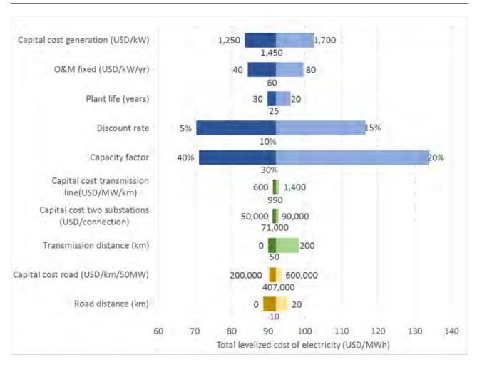
FIGURE 38: Total levelized cost of electricity (LCOE) sensitivity analysis for wind.
