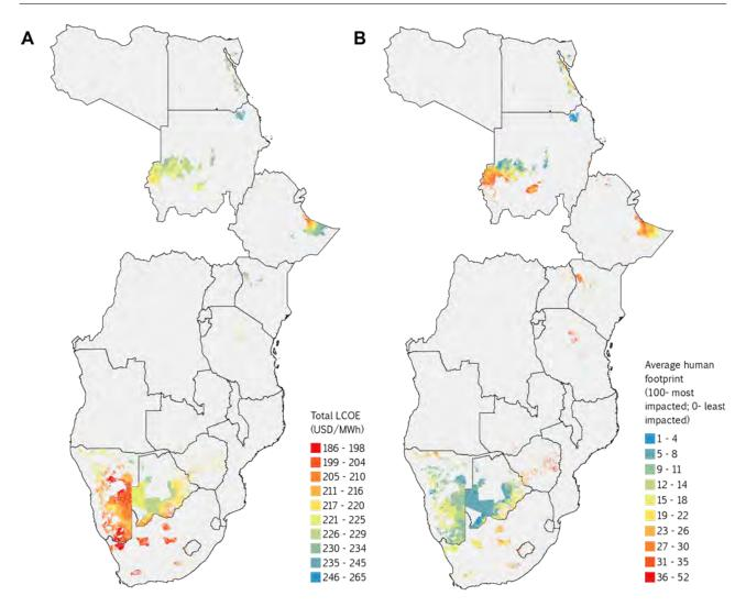
**FIGURE 28:** Comparison of total levelized cost of energy (LCOE) (A) and human footprint score (B) for solar CSP zones.
