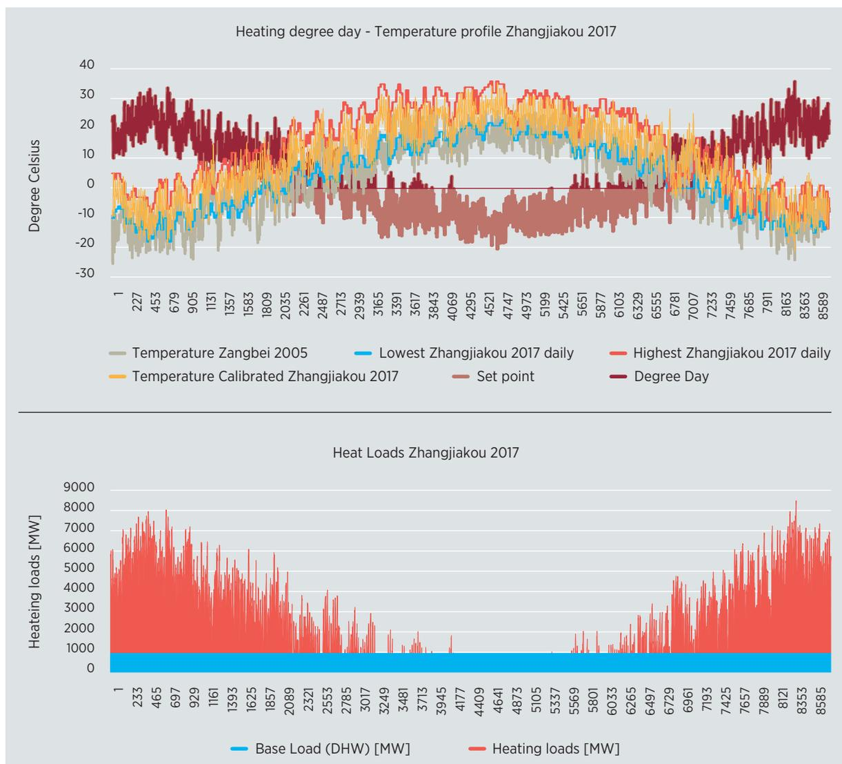
Note: The heat load variabilities for space heating are calibrated with Zhangjiakou's measured total loads. The base loads for domestic hot water are represented in blue.
