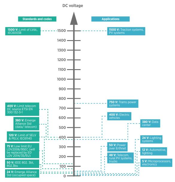
Note: SELV = safety extra-low voltage; PELV = protected extra-low voltage; LDV = laser Doppler vibrometer. Based on: (Rodriguez-Diaz, et al., 2016).
