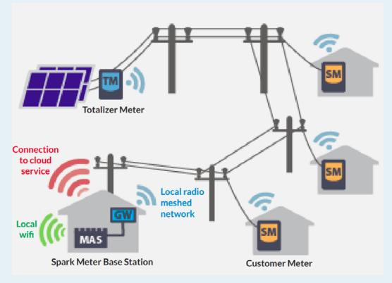
Note: TM = totaliser meter; MAS = SparkMeter base station; SM = customer meter. Source: (SparkMeter, 2019a).
