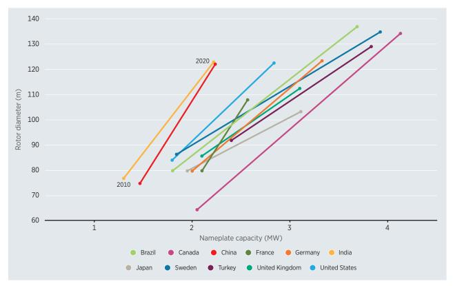
Figure 2.2 Weighted-average osnhore wind rotor diameter and nameplate capacity evolution, 2010-2020
