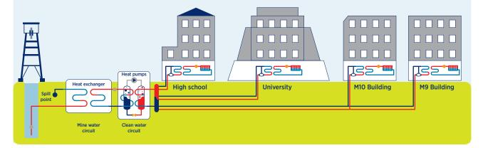
Figure 12. Abandoned coal mines: Barredo Colliery district heating project (Mieres), Asturias, Spain
