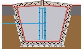
Borehole thermal energy storage (BTES)
