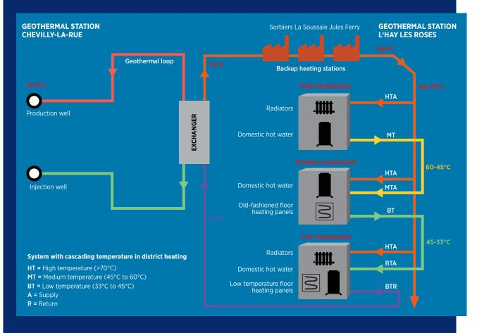
The Île-de-France subsurface is rich in geothermal energy. The utility SEMHACH operates in the Paris suburban municipalities of Chevilly-Larue, L'Haÿles-Roses and Villejuif and implements a cascading multi-temperature district heating system, where five different temperature levels exist, including the transmission pipe temperature.
