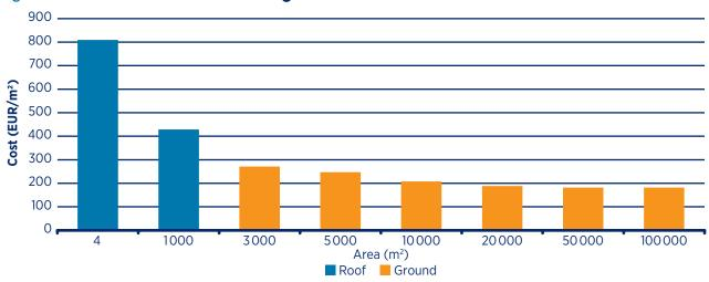
Figure 13. Cost of roof-mounted and ground-based solar installations in Denmark
